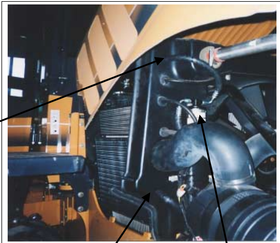
1 1/8" hole drilled in plastic shroud for 13/32" hose
