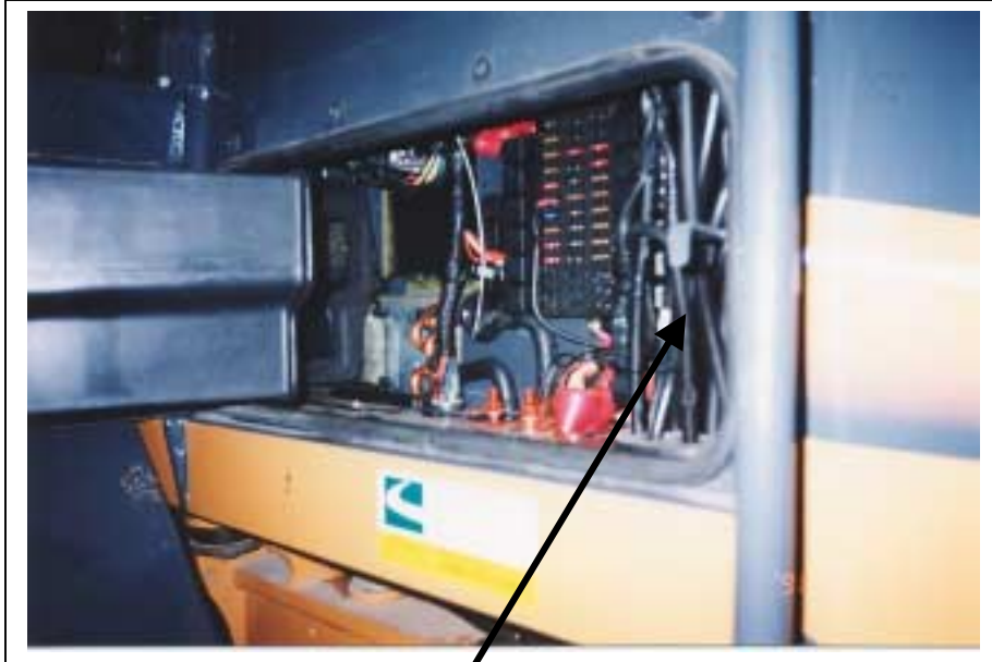
Clutch wire in electrical compartment on right of cab. Run over to the thermostat keeping clear of the filter intake cover.
