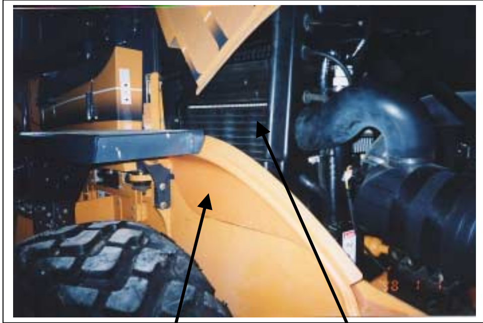
Removable fender well back in place.
